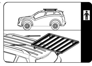
With the help of a friend, flip the rack over, right side up and place it onto the rails of the vehicle.
