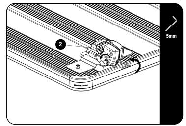
Unlock the Feet and loosen the clamps using a 5mm Allen Key.
