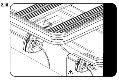
After all the feet are tightened remove the key and store in a safe place.
