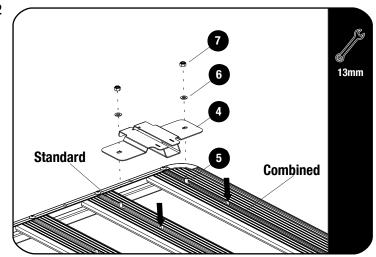
Flip the Rack so that the bottom of the Rack faces up. Insert two M8 x 16 Hex Bolts (Item 5) into the Combined slat and Standard slats machined slots as shown.
